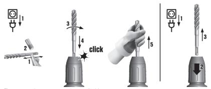
Fit or remove the accessory tool, as applicable.
