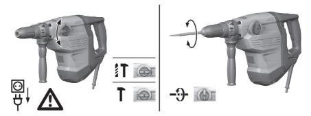
Set the function selector switch to the "Chiseling" position T.
