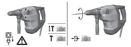
Set the function selector switch to the "Hammer drilling" position
