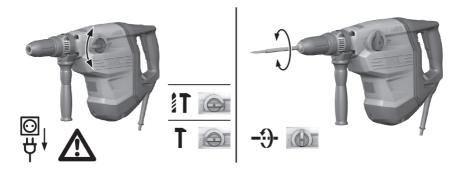
Set the function selector switch to the "Hammer drilling" position and insert the mixing paddle into the quick-release chuck.
